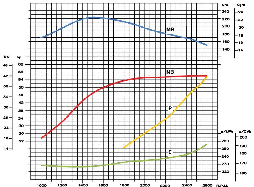
— MB — Torque curve (NB curve)      — P — Propeller demand curve
